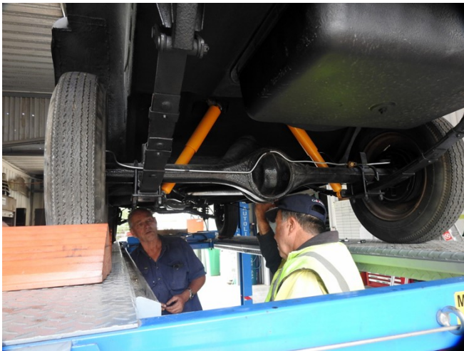
Brian Tucker's FJ Holden. Motor and gearbox in. Bob and Mark fit the tail shaft.
