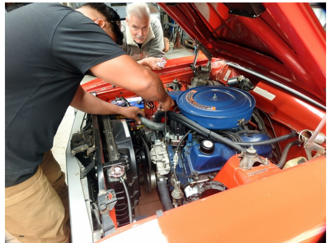
Jon Jon Ramirez installing a new thermostat in his 1972 XA Ford Falcon GT.
