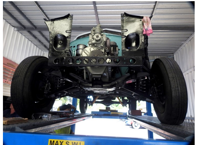
Brian Tucker's FJ Holden. Motor and gearbox in. Bob and Mark fit the tail shaft.
