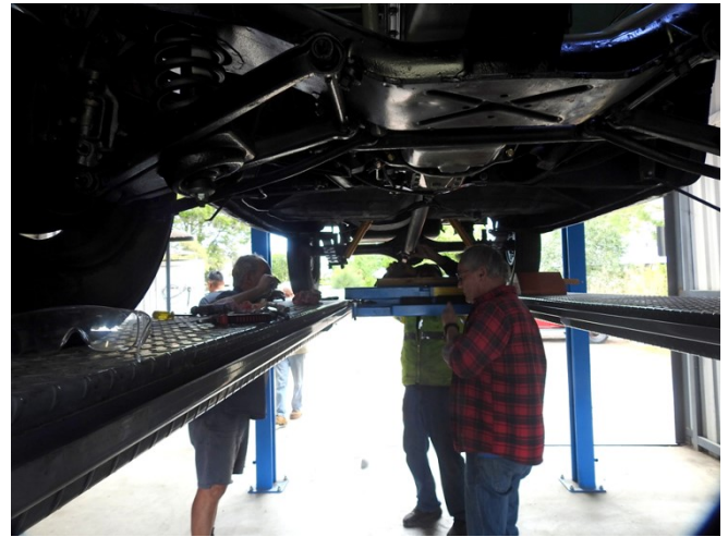
Brian Tucker's FJ Holden. Motor and gearbox in. Bob and Mark fit the tail shaft.
