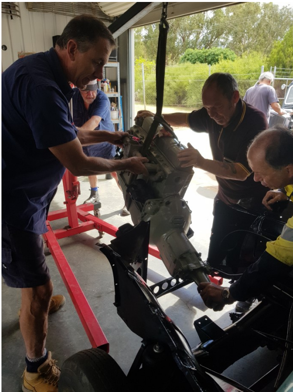
1954 FJ Holden, long time resident of the workshop getting engine and gear box fitted .
